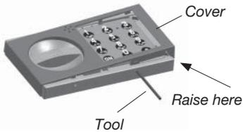
Press tool into the right hand or upper (in case of vertical installation) hole on the bottom edge of the control unit until the catch is released. Keep the tool pressed down whilst the cover raising carefully.
