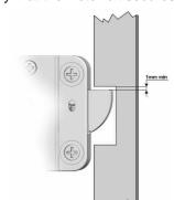
In the LOCKED position the distance between the RotoBolt bolt and the boltwork part that is moving the lock bolt should be approximately 1 mm.
