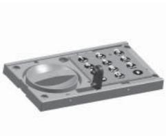
Pull out the battery clip for the emergency supply by about 1 cm and clip in a 9-volt block battery. Open the lock with a valid code, remove the block battery from the clip and replace the discharged battery in the lock case.
