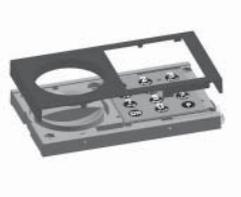
Replace the cover and press down until all four catches are engaged. Check that the lock functions correctly whilst the safe is still open.
